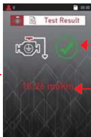
Test result indicating the ground connection is good.
